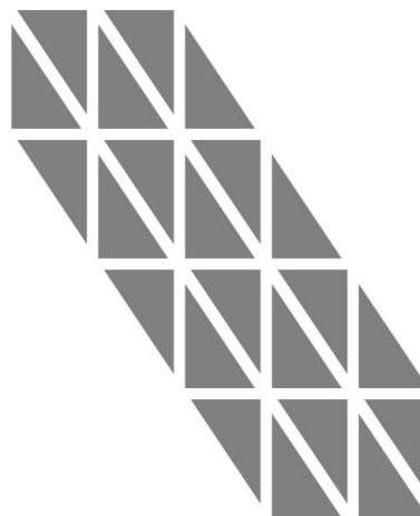
Figure 14 Cartoon of a crystal structure comprising two identical particles (triangles) per unit cell, but where the cell occupancy of the particles varies along the surface of the nanocrystal.
